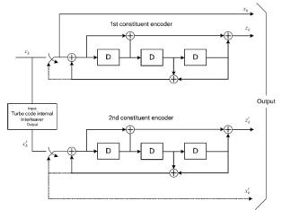
Figure 5.As can be seen in Figure the output of the LTE Turbo encoder consists of three parts, a systematic bit and two parity bits. The systematic bit is the untouched input bit.
