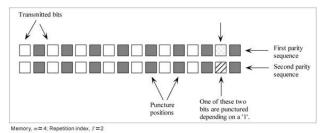
Figure 4. Figure shows the positioning of the puncturing at the transmitter for the dual-repeat-punctured superorthogonal convolutional turbo codes.
