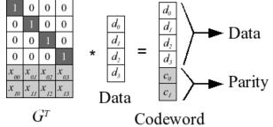
Figure 3.Shows Reed-Solomon coding for k=4 and m=2. Each element is a number between 0 and 2w-1.
